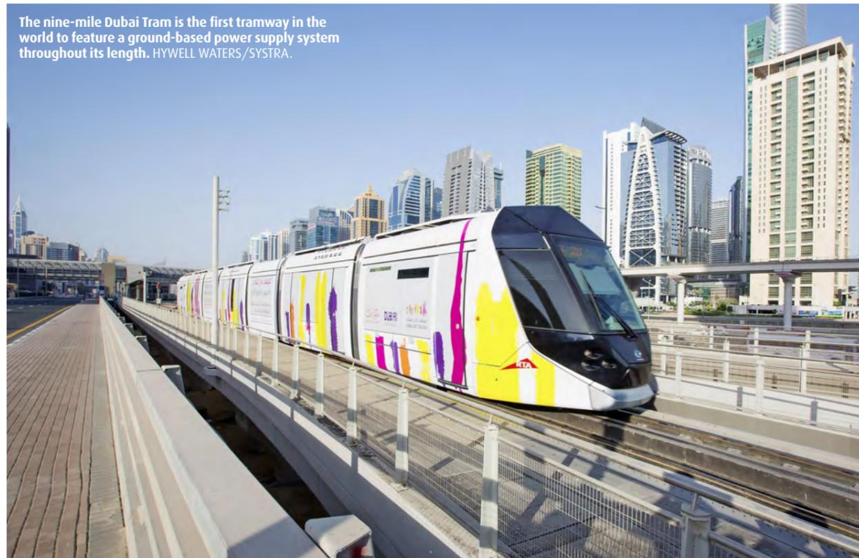
The nine-mile Dubai Tram is the first tramway in the world to feature a ground-based power supply system throughout its length. HYWELL WATERS/SYSTRA.
